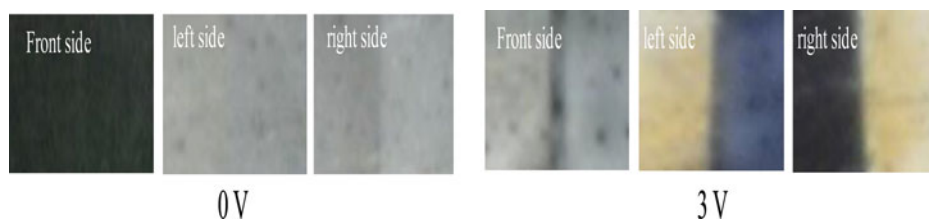
Figure 6. Photo images taken at the front side, left side, and right side of the fabricated LC cell.
